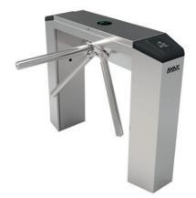
Industrial parts are used for 24 hours continuous application and durable. Body and arms are stainless 304 quality steel. It has a dry contact relay of 12 volts or 24 volts. The passing width is about 55 cm. Passing intensity is 35-50 persons per minute. Operating frequency 50-60 Hz Dimensions are 1200 x 280 x 980 mm / Weight: 52 kg
