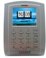
TCP/IP Connection. CLOUD Supported Card Reader. It has a capacity of 50,000 users. It can recognize 50,000 cards or passwords. It has a capacity of 160,000 logs It allows to pass through password or card. The card it reads can be launched from CLOUD to a computer in a different location. Width: 9 cm x Height: 12 cm x Depth: 4 cm. The keys can be programmed as desired.
