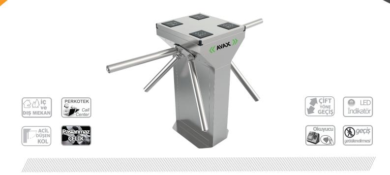
Avax D100 Drop Arm Turnstile allows both entries and exits at the same time. Thanks to the Emergency Dropping Arm feature in both directions, it provides fast and safe evacuation by going down in case of a power failure, signal from the fire alarm system or emergency situations. With the Emergency Button connection you can release all passes. Button connection can be made for guest or VIP passes. By connecting the counter on the turnstile, the total number of passes per day can be obtained.
