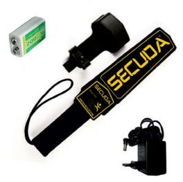
Frequency / Voltage: 22 KHZ / 9 V Dimensions: 410 x 85 x 45mm / Weight: 409 gr. Distinguish between ferrous and other metals. Audible, illuminated and vibrating warning Sound and light warning in low battery. Ability to adjust sensitivity. Leather-covered, easy to use and ergonomic, healthy design. (with battery and charge adapter)
