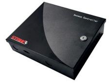
24/7 continuous operation / With 12V 2A battery 16 Wiegand card readers can be connected It has 2 pcs of RS-485 ports It has 10 Mbit Ethernet-TCP / IP interface Power supply 12V DC min. 1 A / Voltage control LEDs It has 10A NC / NA relay output. Can keep 100,000 events in memory. In the same network, 256 ad panels can be used and 4,096 card readers can be controlled at the same time. / It has 1 pcs of RS-232 port. LED monitoring for optical interface.
